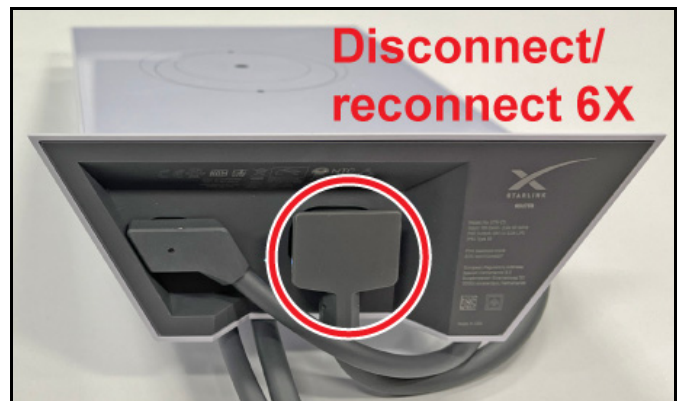
Figure 7: Starlink Gen 2 Router Power Cable Connection
