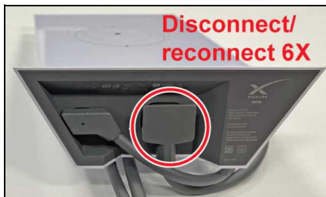
Figure 16: Starlink Gen 2 Router Power Cable Connection
